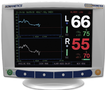
Figure 5. INVOS™ monitor. The green vertical five-bar signal strength indicators are shown for each INVOS™ recording channel. Signals with a stable reading of more than one bar are sufficiently strong to permit reliable monitoring. Large font numbers display the momentary rSO_2 values for each channel, which are updated every 5 seconds. Mid-size font numbers display the baseline values. Red numbers reflect an oxygen debt alarm, and the small font values display the percentage change from baseline.
