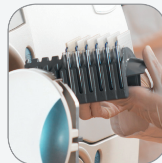
VITEK 2 Compact: Cards inoculated inside instrument and manually transferred from filling door to loading door for processing
