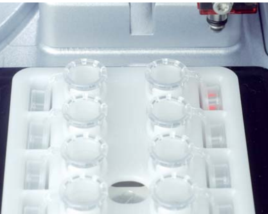
Figure 2. Hands-free sample lysis. The integrated shaker enables fully automated lysis of up to 12 samples.
